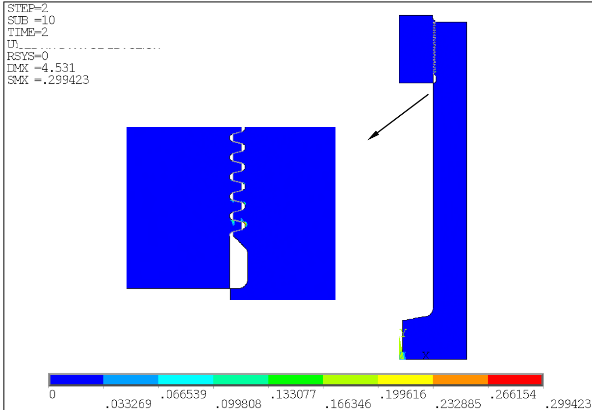
Figure 12 – E-KD-2.2.2-3 – Elastic-Plastic Strain Limit Ratio Results for Local Failure Analysis Results at 57,600 psi
